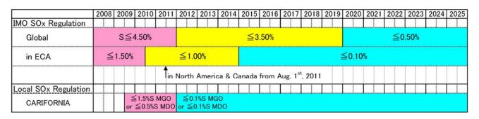
The low sulfur fuel mostly means the usage of distillate fuel oil such as MGO (Marine Gas Oil) and MDO (Marine Diesel Oil). This guideline is prepared for general guideline using the distillate fuel on Mitsui MAN B&W engines.
